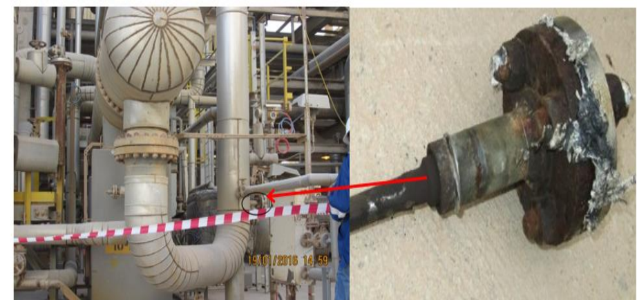
Failure Analysis of Flange Weld Socket Assembly in a Methanol Plant ( CNG Leakage at 28 bar Operating Pressure)
